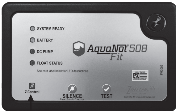
Figure A, FIT Controller
