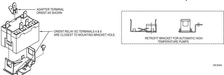
Select the relay mounting bracket required based on pump model using drawings above as a guide. Snap relay into mounting bracket. Be sure relay tabs engage mounting bracket ears on both sides. Secure relay to housing with screw provided. Reconnect wires per wiring diagram available on service part sheet.
