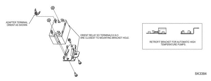
Select the relay mounting bracket required based on pump model using drawings above as a guide. Relay does not snap into mounting bracket, it is secured to the bracket with screws and nuts. Secure relay to housing with screw provided. Reconnect wires per wiring diagram available on service part sheet.
