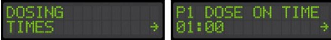
If the “DOSING TIMES” screen does not display, the system might be configured for demand dosing. Check in the “Advanced Settings” shown below that the system is in time dose mode.
