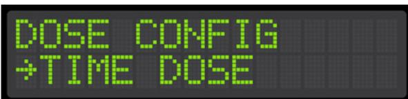
If you selected Time Dose Mode, the system will ask if a Peak Timer should be enabled. If enabled, FLT 3 will become a Peak Timer Override input. When activated, this input will load in the “Peak” dosing times. These Peak times can be programmed to dose more aggressively to keep up during high demand times.
