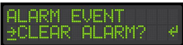
Note that if the alarm immediately re-activates and the buzzer activates again, this means that the alarm condition is still present and the system cannot clear the alarm. If this happens, check for the source of the alarm.
