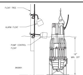
Use the diagram above to secure the float switch properly and obtain the proper tether to customize the on-off cycle to each application. Note the minimum off level shown above. On Prepackaged Systems, the tether length is set at 5".
