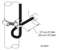
**Note:** Failure to keep within proper tether limits may prevent reliable switch operation.
