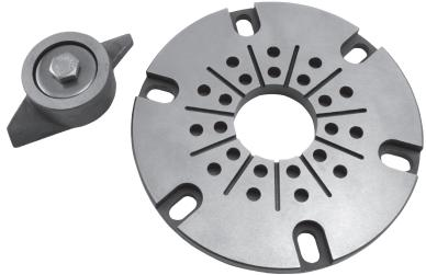
To remove cutter: Heat the center bolt to 350 °F to loosen Loctite® thread sealant.
