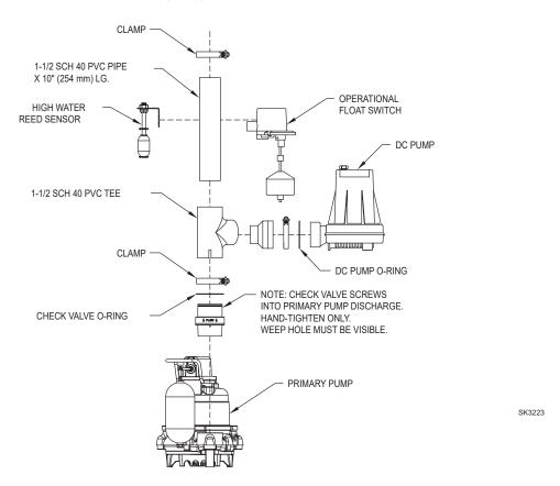
**▲ IMPORTANT** To minimize risk of air lock, intake of DC pump must be set <u>above</u> intake of primary pump.
