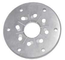
Grind the Star Cutter and Disc seen here to a 32 microfinish. Surfaces must be flat to within 0.001" T.I.R. Gap must be between 0.004" and 0.008" on these parts.
