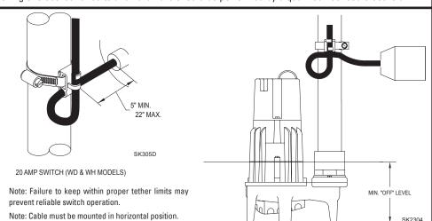
Models WD & WH are fully automatic. A float switch is included and factory wired in the pump circuit to provide automatic operation once the float switch is secured properly to the outlet pipe. Use the diagram above to secure the float switch properly and obtain the proper tether to customize the on-off cycle to each application. Note the minimum off level shown above. On Prepackaged Systems, the tether length is set at 5".
