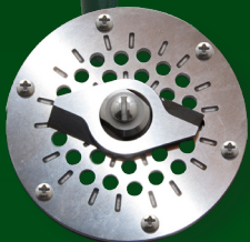
Grinder blade and cutting plate
