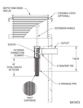
Zoeller Pump Company septic tank effluent filters are designed to protect all downstream components from solids. Every filter comes standard with bypass protection which keeps the filter working, even during cleaning!
