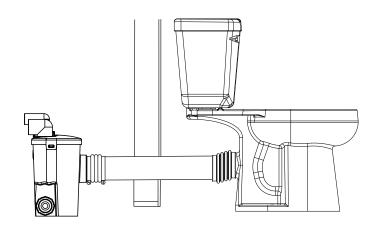
Connect the rear discharge toilet to the front inlet of the Qwik Jon® Premier via hose clamps. Ensure the connections are according to local, regional, and state codes.
