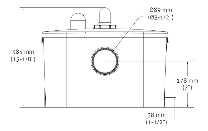
Connect the desired inlet pipe from other fixtures to the side inlet(s) of the Qwik Jon® Premier. Use a 1-3/4" (44 mm) hole saw to cut hole in side inlet(s)
