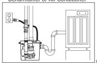
Applications include: laundry tray pump, wet bar sink, lavatory, air conditioning condensate or dehumidifier water removal. It can also be used in conjunction with dishwashers and garbage disposal applications.
