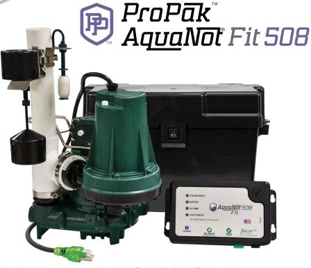
ProPak 508-0015 with primary pump M53® with Zoeller LED plug shown. System includes: Model 53, 63, or 98 primary pump with LED plug / Aquanot Fit 508 Z Control enabled controller, Model 508 Aquanot®, 12 Volt DC backup system with DC pump, check valve, float switch(es) and piping / Plumbed in 1-1/2" (DN40) Sch. 40 PVC pipe.
