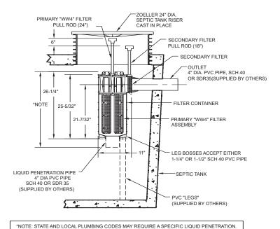
FOR EXAMPLE, 25% - 40% INTO THE LIQUID DEPTH OR 9" OFF THE TANK BOTTOM.
