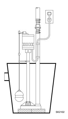
NOTE: This unit is designed for indoor applications where the motor is mounted above the pit cover and protected from water, water spray, and high humidity. Pump is not intended for use with flammable liquids.
